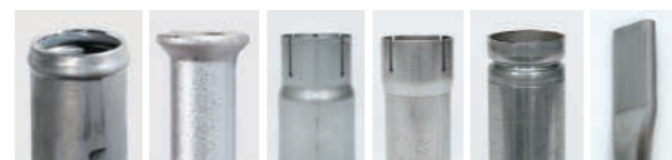
▲ Beading ▲ W flare ▲ Tube reduction ▲ Tube expansion ▲ Spinning ▲ Crush
