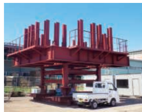
▲ 350ton load testing stand
